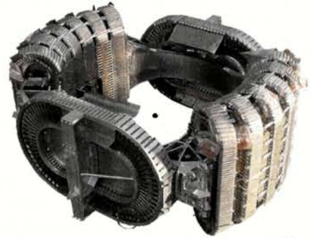
AMS - a 1.1 m clear bore actively-shielded dipole magnet for use in space
