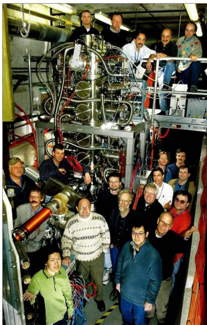
The polarized hydrogen jet target at RHIC surrounded by some of the members of the development team. (Courtesy Roger R Stoutenburgh BNL Photography and Graphic Arts.)
